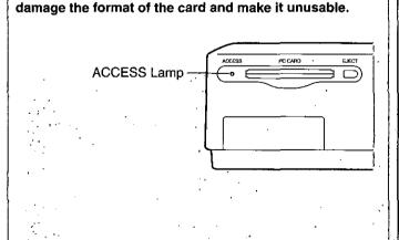
Never pull out or insert the card while the ACCESS Lamp
